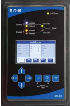
ATC-900 Main Screen Shows Current Values
