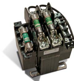
Fig 6. Eaton control power transformer with built-on fuseholders. The transformer is protected by Eaton Bussmann Series fuses, primary by class CC type FNQ-R, and secondary by Midget Type FNM. Protective cover for fuses and terminals are available as accessories.
