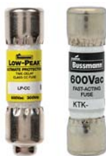
Fig 5. Left side fuse is rejection type class CC, right side fuse is a Midget fuse. The dimensions are the same for both types, 10,3x38,1 mm. One of the contact ferrules on the class CC fuse is equipped with a rejection key, in this case a tap. The design prevents installation of a Midget fuse in a fuseholder intended for class CC fuses.
